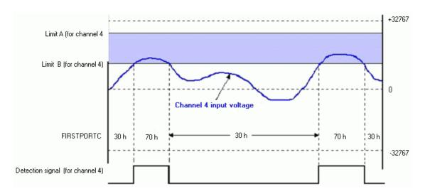
Figure 26. Analog inputs with setpoints update on True and False
